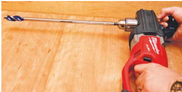
▲ There's an easily operated push-through forward/reverse switch
